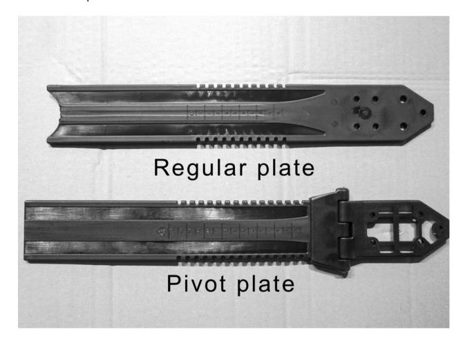
The Pivot version has a hinge built into the plate where most of its flexing takes place. This means the pivot plate has an easier flex (in regard to touring), especially in cold weather when plastic stiffens.
